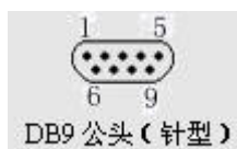
Figure 4. RS232 Pin Defination(Male/Needle Type)
