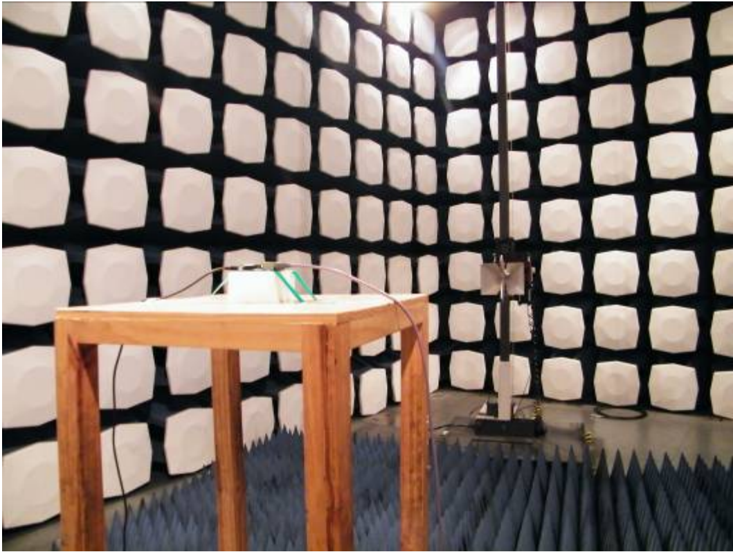
Picture 2 Radiated Spurious Emissions Test Setup
