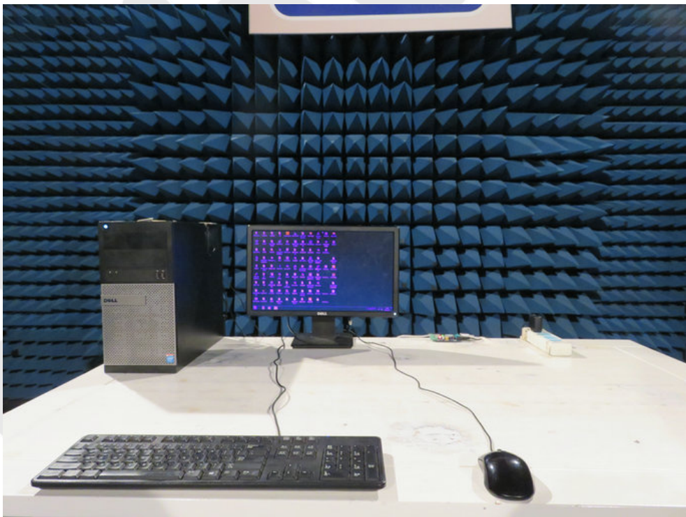
Photo of RF Field Strength Susceptibility Test
