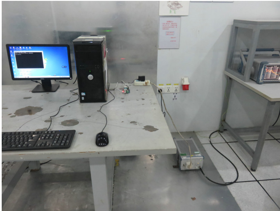
Photo of Conducted Emission Test
