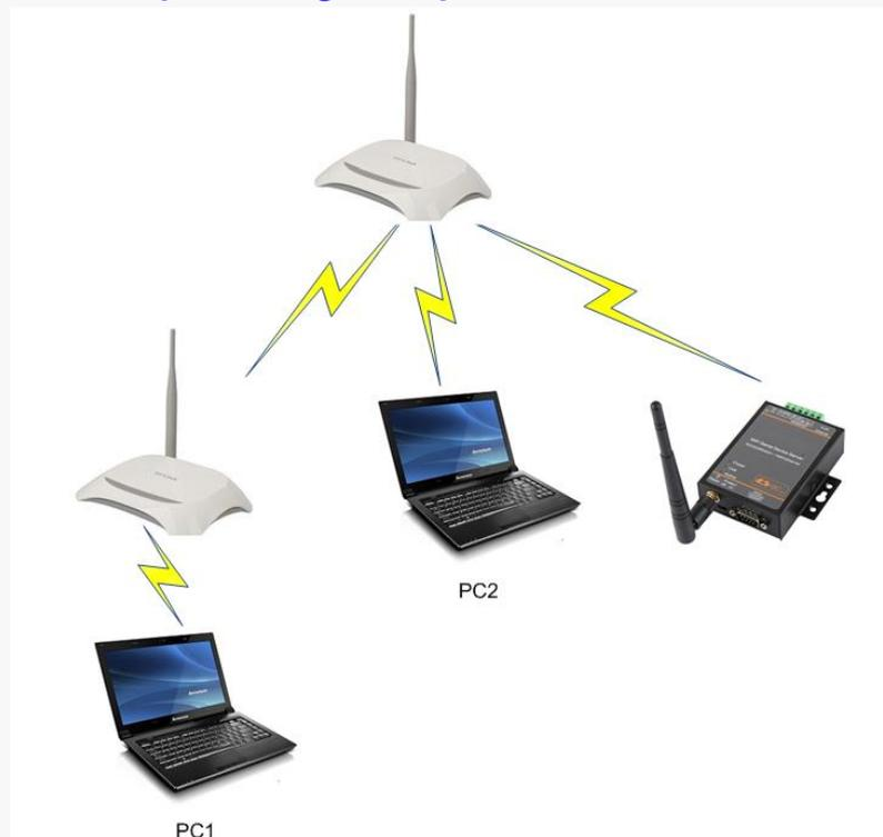
**b ) LAN environment, set the IP of the device but may not be in the same network segment with the router, through IOTService broadcast search function can be modified to the same network segment and then configure.**
